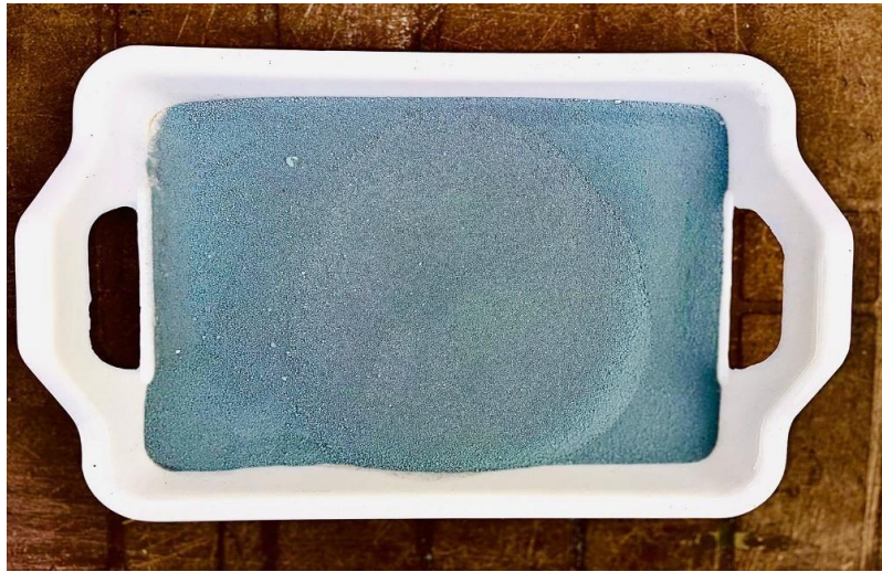
Figure 3: Silica Fume Sample
