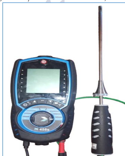
Figure 3. Flue gas analyzer
