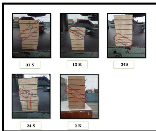
Figure 4: Cracks produced during UCS with wrapping of iron wire
