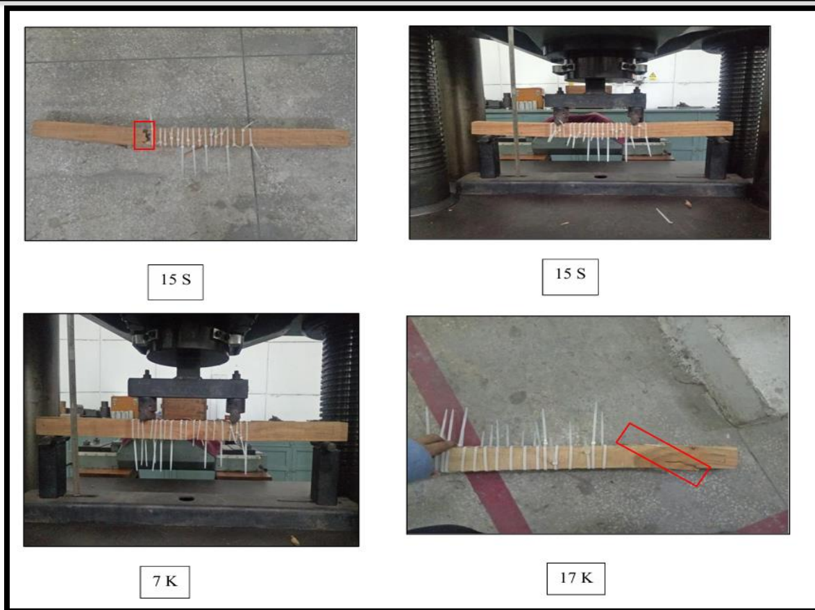
Figure 18: Cracks produced during flexural testing samples covered with plastic tie
