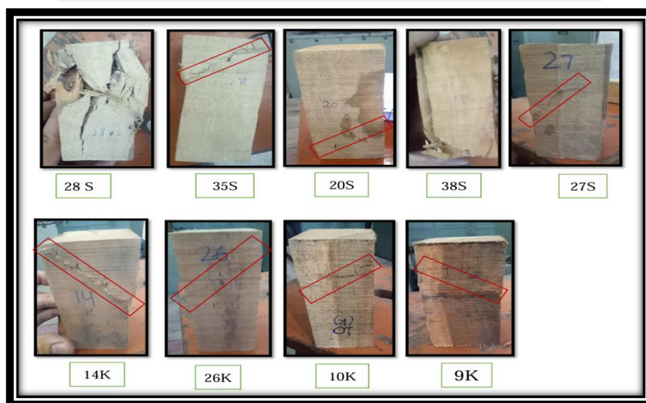
Figure 2 Samples for UCS with wrapping tie plastic
