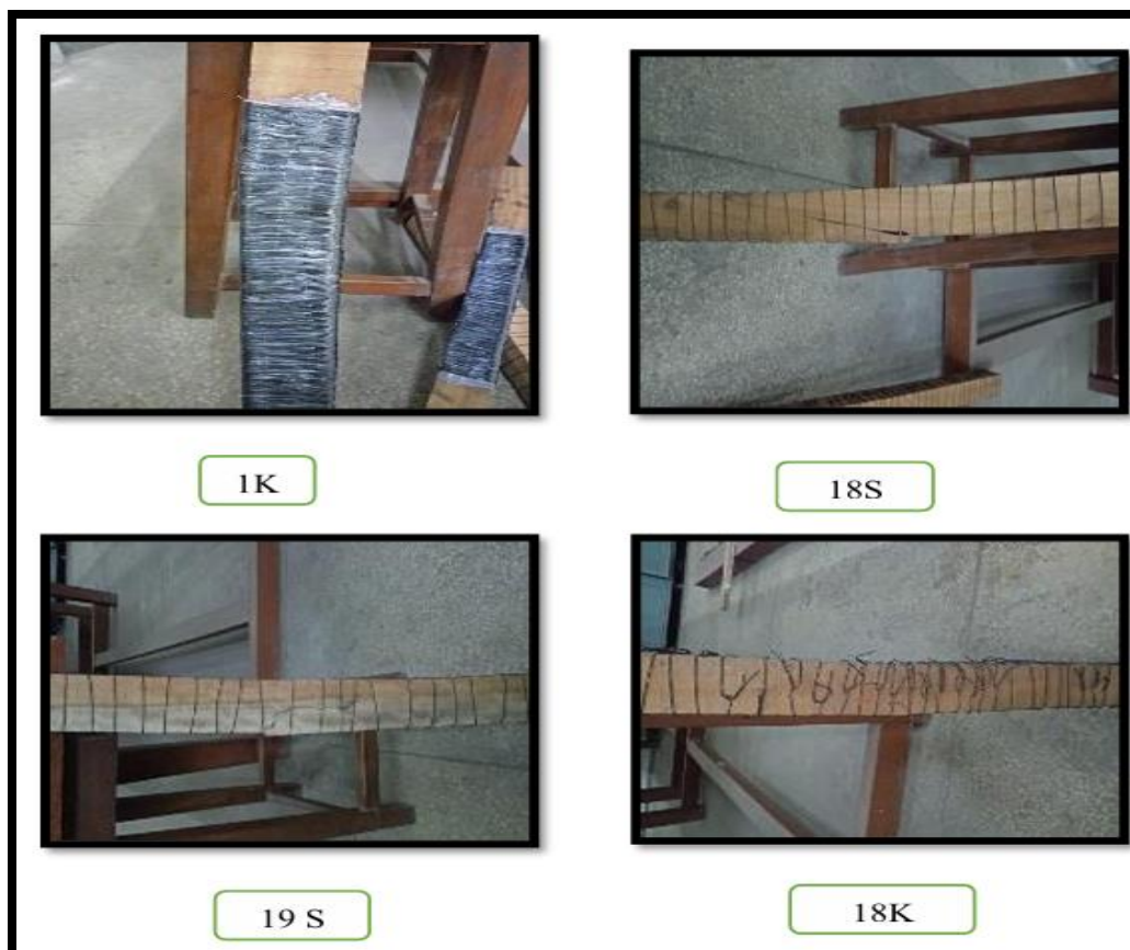
Figure 22: Cracks produced during the fractural test of sample wrapped with iron wire, (19S, 18S, and 18K), and (1K) sample is wrapped with sika 230
