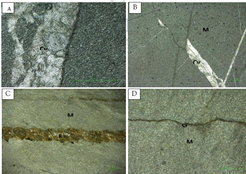
**Figure 3.** Photomicrographs (XPL) of the studied limestone unit of the Darwaza Formation (A) showing calcite vein (Cv) and micrite (M) and dolomite (Dl); (B) Weakly developed stylolite (St) and calcite vein (Cv); (C) Ferruginous material (F) and micrite (M); (D) A well-developed stylolite (St).
