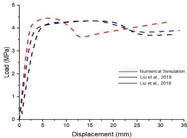
Figure 5. Experimental vs. simulated load-displacement curves (for void-controlled precast CFST columns).
