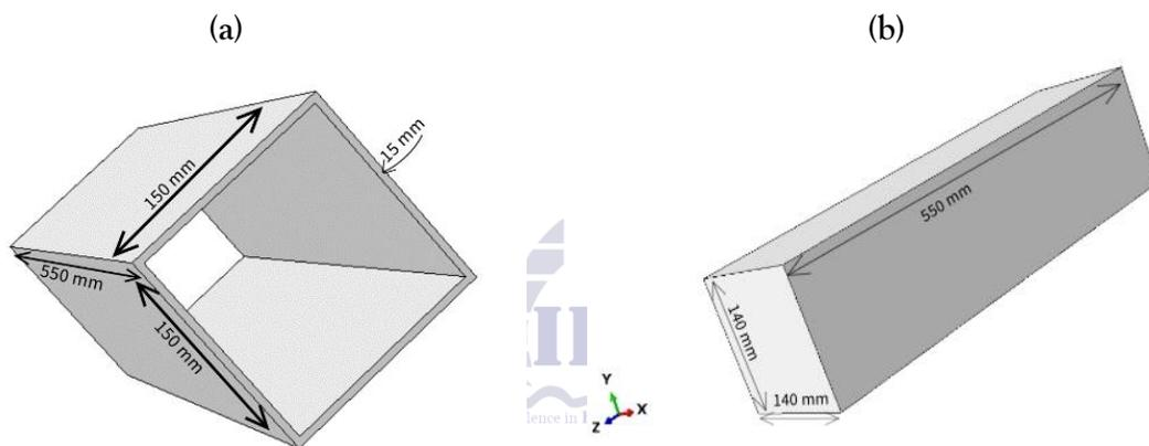
Figure 1. Geometry of Materials (a) Steel Tube (b) Concrete
