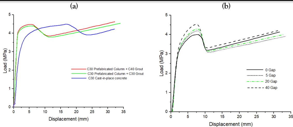
Figure 8. Load vs. Displacement curve (a) C30 concrete with different C30, C40 Grout (b) 0, 5, 20, 40 width gap curve
