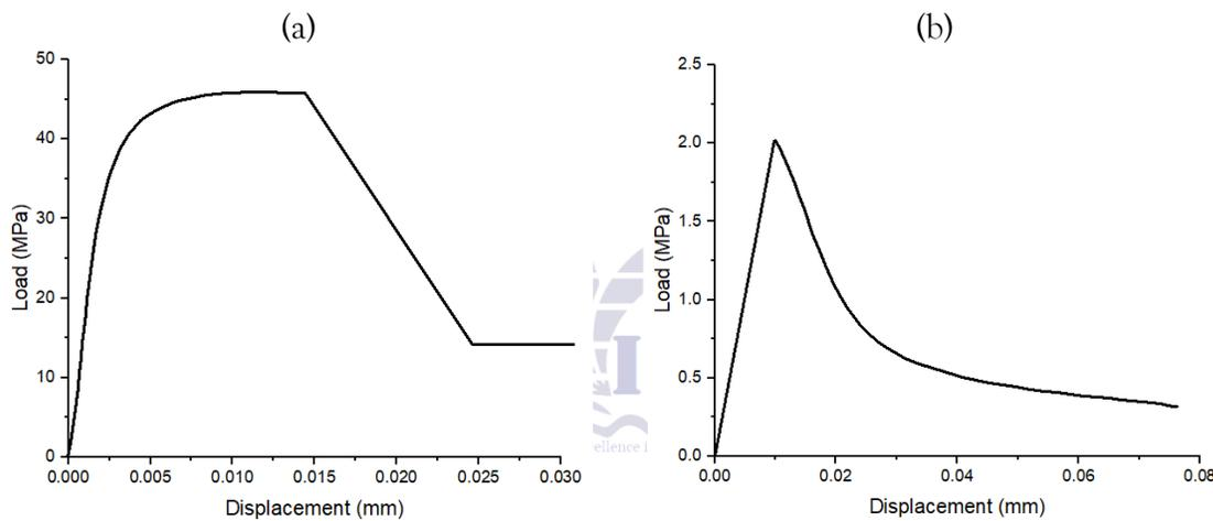
Figure 4. Constitutive Model of Concrete (a) Compression model (b) Tension model
