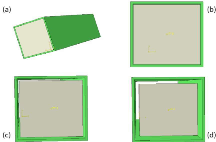
Figure 6. Numerical simulation results for different gap widths: (a) 0 mm gap, (b) 5 mm gap, (c) 20 mm gap, (d) 40 mm gap
