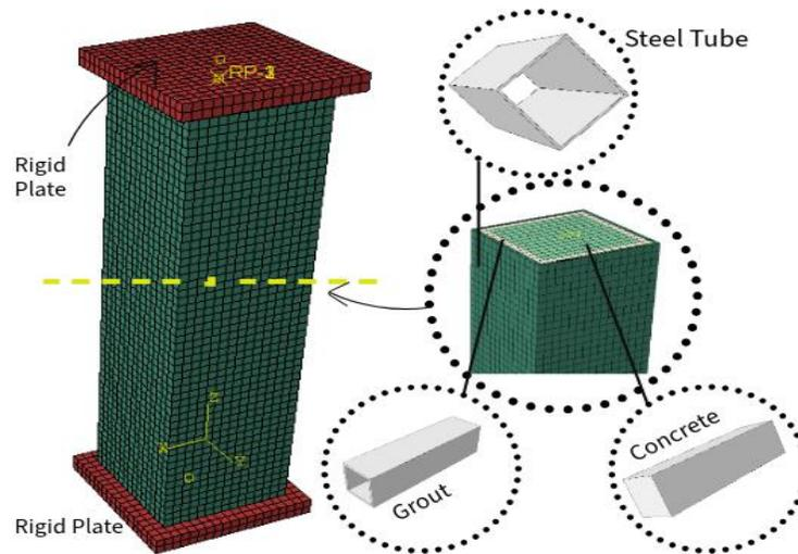
Figure 2. Advanced meshing strategy (emphasizing void geometry parameterization and material interfaces).
