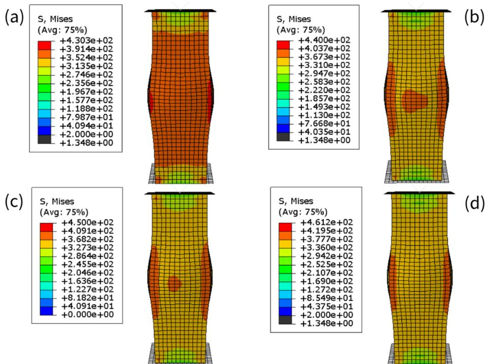
Figure 7. Von Mises stress distribution for varying gap widths (a) 0 mm, (b) 5 mm, (c) 20 mm, (d) 40 mm
