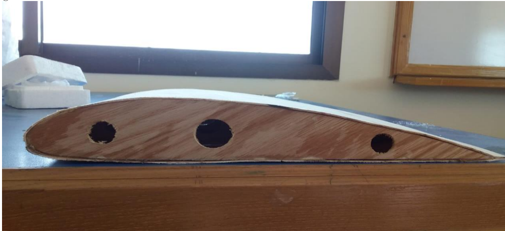
Figure 10 Prototype hardware of 4415 cambered airfoil
