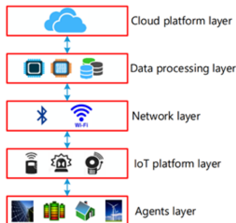
Figure 6: IoE Communications Network Layers – This figure shows the four layers in the Internet of Energy (IoE) communication network, including the Agent Layer, IoT Platform Layer, Network Layer, and Data Processing Layer, highlighting how data flows between devices and the cloud for energy management.
