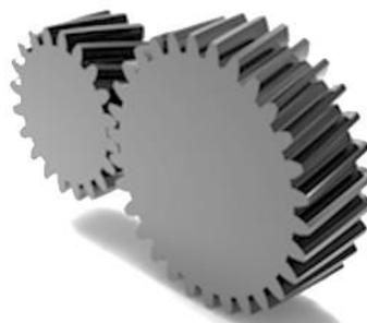
Fig. 4. Two-gear reduction assembly diagram, with a 2:1 speed reduction and increased torque from the motor to the wheel axle.
