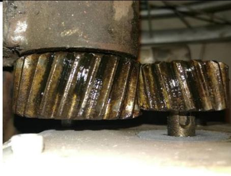
**Fig. 5. Installed gear assembly with helical gears, transmitting power from the motor to the wheel and increasing torque for smooth operation.**
