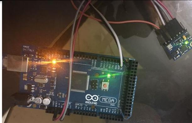
Fig. 9. Arduino Mega connected to the GY-87 IMU sensor (right), reading head tilt data via I<sup>2</sup>C for motor control decisions.
