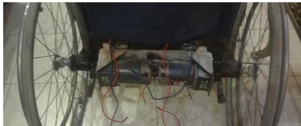
**Fig. 6. Bottom view of the motor installation. Two DC motors are mounted on a metal plate under the seat, connected to the H-bridge driver for efficient power transfer**
