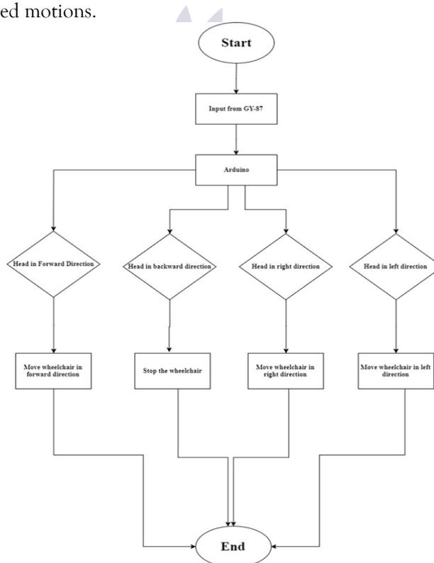
Fig. 11. Flowchart of tilt-based motion control implemented on the microcontroller.
