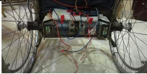
Fig. 7. Electronic control unit with Arduino Mega 2560, IMU sensor, relay circuits, and dual 12 V batteries for power.
