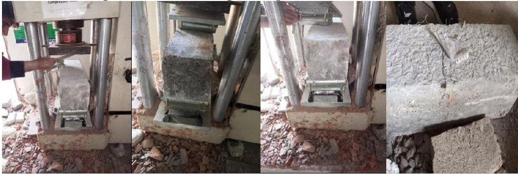
Figure.16 Flexural Strength Test
