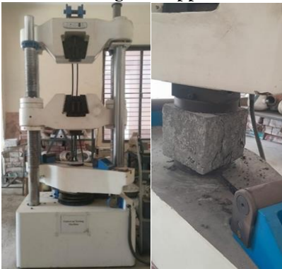
Figure 14: Cube Being Tested for Compressive Strength
