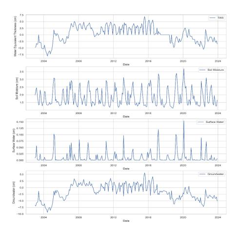
Figure 2 | Variation in TWS, soil moisture, surface water and groundwater storage.
