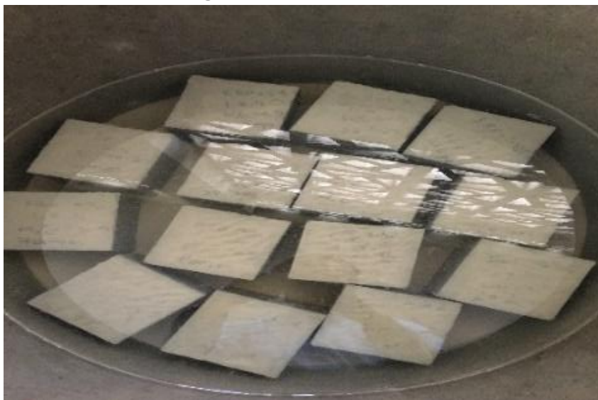
Figure 9: Specimens kept in water tank for curing
